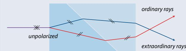
The Nomarski prism consists of two birefringent crystal wedges cemented together at the hypotenuse. One wedge is a Wollaston wedge, the second wedge of the prism is modified by cutting the crystal so that the optical axis is oriented obliquely with respect to the flat surface of the prism
