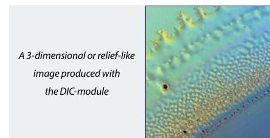
brightfield techniques has greatly improved. These relief-like images are ideal for surface inspections of wafers, LCD screens, etc
