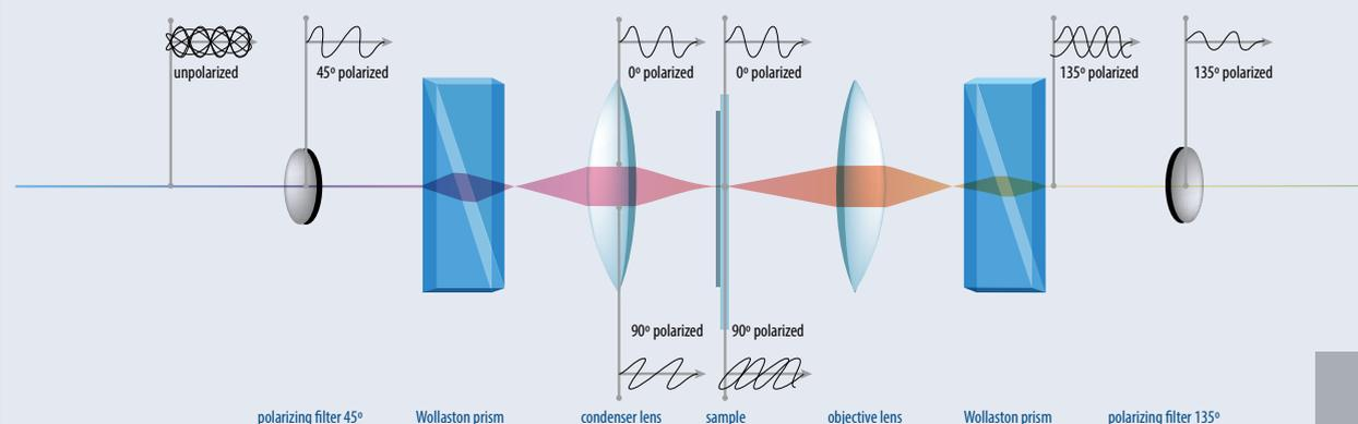
By passing a second Nomarski-modified Wollaston prism, the spatially shifted polarized light is recombined. These recombined light rays pass through a second polarization filter that blocks useless direct transmitted light. The interference of the two rays is sensitive to the optical path difference and by introducing an adjustable offset, the contrast is proportional to the path length so that the heights
