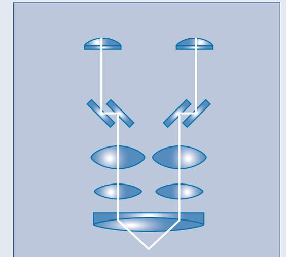
Two parallel optical trains share a common main objective and generate two images under a small angle
