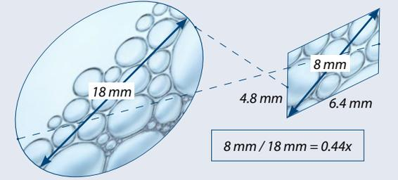
Furthermore, the circular eyepiece FOV is much larger than the camera FOV and thus the microscope FOV must be "reduced" with a so-called "relay" lens or "photo-adapter" to fit the camera FOV. However - in order to avoid vignetting (dark shadows in the corners of an image), the circular microscope FOV must just be projected outside the image sensor area. Subsequently the camera FOV will always be smaller than the microscope FOV by 50 to 60%
