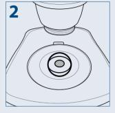
Put a specimen on the stage plate
