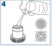
Clean the lens by using the tip of the cotton swap or lens paper\*. When cleaning a large lens surface, wipe with little pressure from the center towards the periphery in a circular motion, do not use zig-zag motion. Discard each lens paper or cotton swap after a single use
