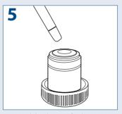
Wait until the cleaning fluid is evaporated, or speed up this process by using pressurized dry air
