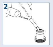
To prevent scratches on coatings and optical glass, first try to remove dirt and dust that sticks to the optical surface with an air-blower or pressurized dry air (oil-free and under moderate pressure version only)
